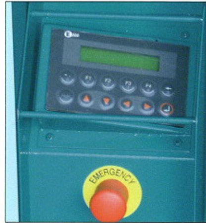
HMI Control Unit
